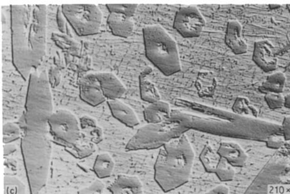
Figure 4 Microstructures observed in chill-cast ingots: (a) Dendritic \alpha -Al solid solution observed in chill-cast wedges of Al-5 wt % Mn; (b) dendritic Al_6Mn in a cellular \alpha -Al solid solution matrix observed in chill cast Al-10 and 15 wt % Mn; (c) primary Al_4Mn in a cellular \alpha -Al solid solution matrix observed in chill-cast wedges of Al-15 wt % Mn; (d) bundles of LT-Al_{11}Mn_4 platelets observed in chill-cast wedges of 18 wt % Mn; (e) and (f) decagonal phase together with some dendrites of Al_6Mn (e) and decagonal and icosahedral phase, (f) observed in chill-cast wedges of Al-10 and 15 wt % Mn, respectively; and (g) and (h) icosahedral phase served in chill-cast wedges of Al-15 wt % Mn.
